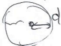
$$P = \text{cte} \Leftrightarrow \Pi \times 4\pi d^2 = \text{cte} \quad \Leftrightarrow \Pi = \frac{\text{cte}}{4\pi d^2}$$
